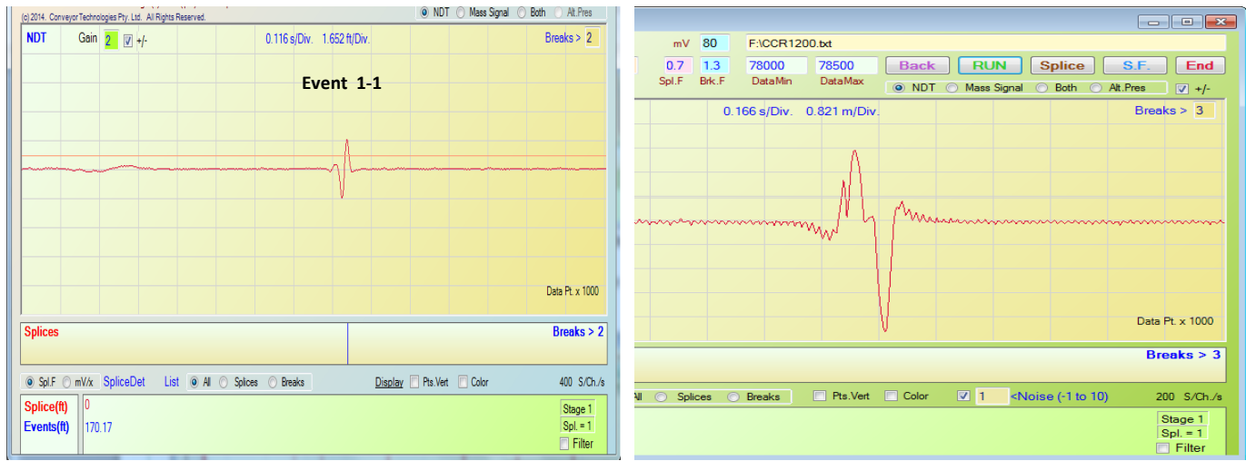
a) Belt scan signals for actual broken cables (0.8 ft. signal) b) Spurious magnetic pockets (3 ft. long signal).
